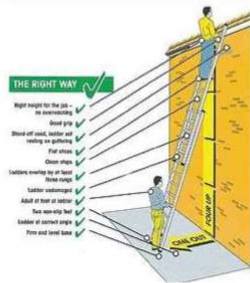
Fig 5-Right way of using a ladder
